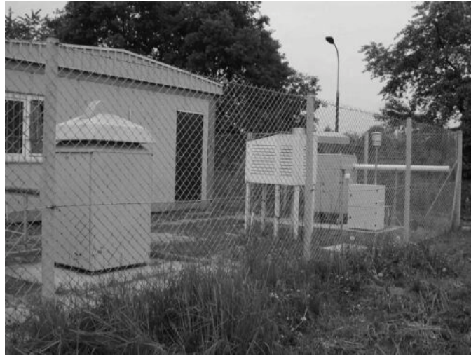
FIG. 3. A view on radiometric station of Institute of Nuclear Physics in Kraków. One of high volume aerosol sampling stations AAS-500 is visible on left side.
