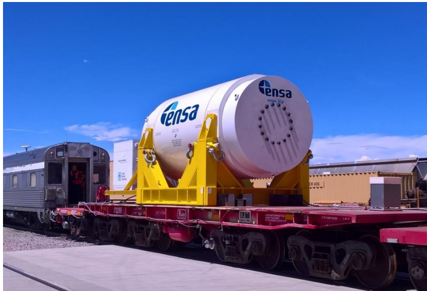
International Multi-Modal Surrogate Spent Nuclear Fuel Transportation Test project in 2017, with ENUN 32P cask
