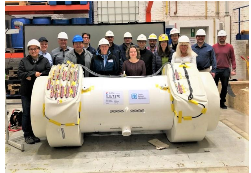
30 cm Horizontal Drop Test in 2018, with 1/3 scale mock up of ENUN 32P cask
