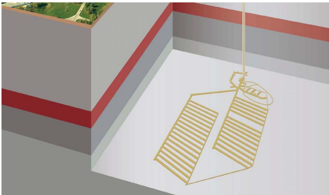
Figure 4-7. Simplified design of the Bruce repository.
