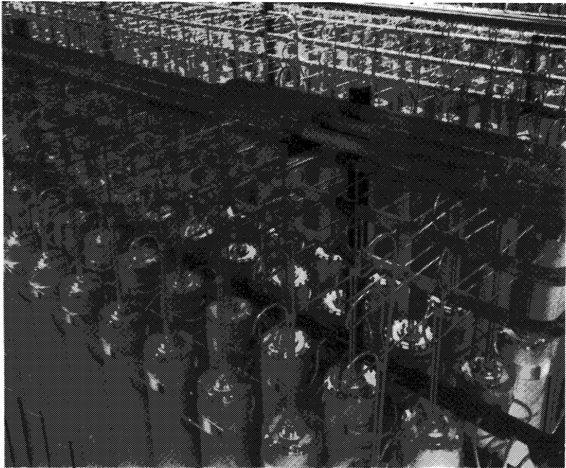
FIG. 3.3. View of centrifuges in a cascade hall of an enrichment plant.
