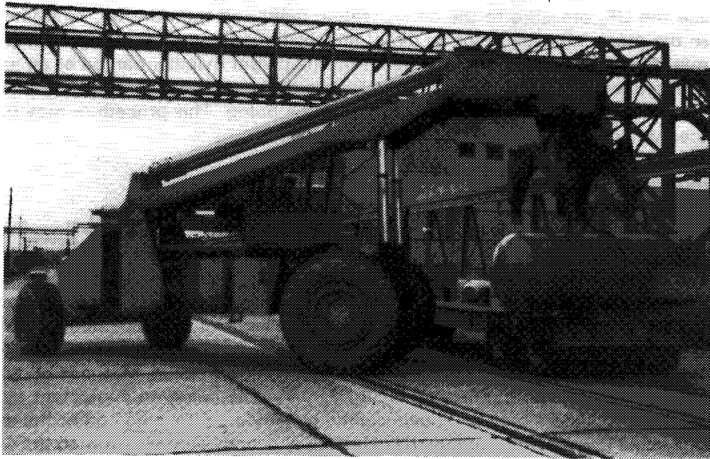
FIG. 3.15. UF 6 cylinder handling equipment.
