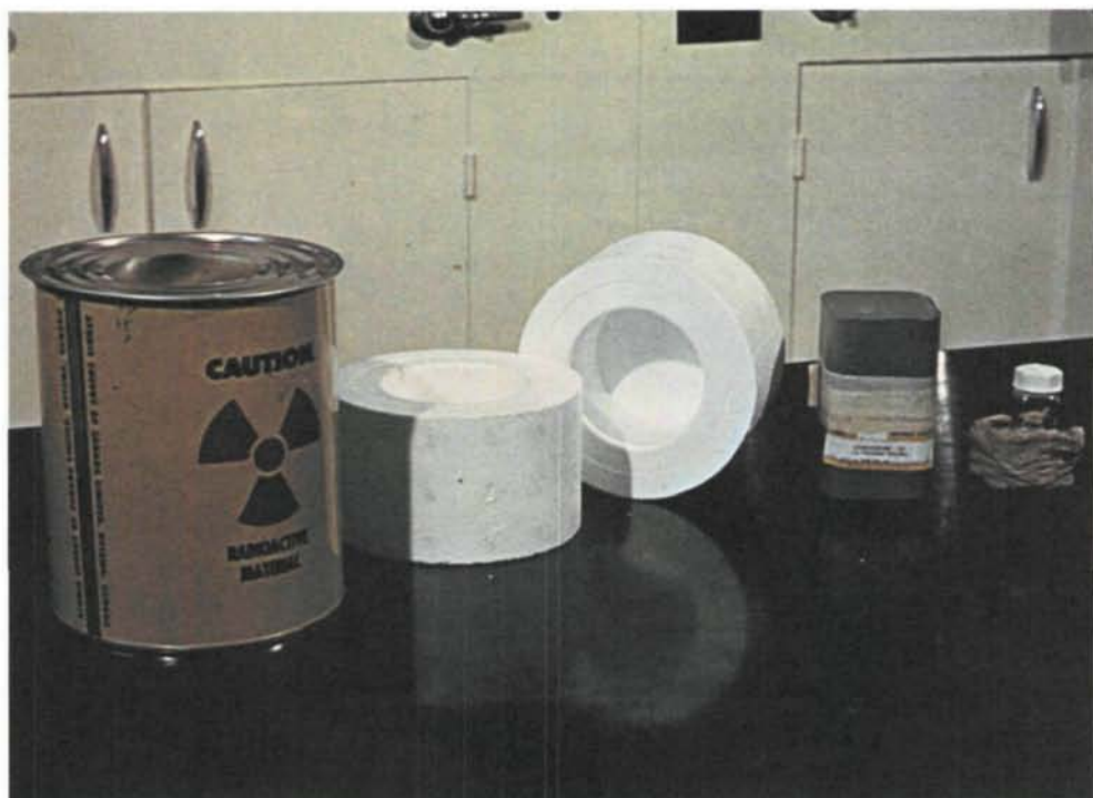
Figures 1a, 1b. Components and assembly of a Type A package.
