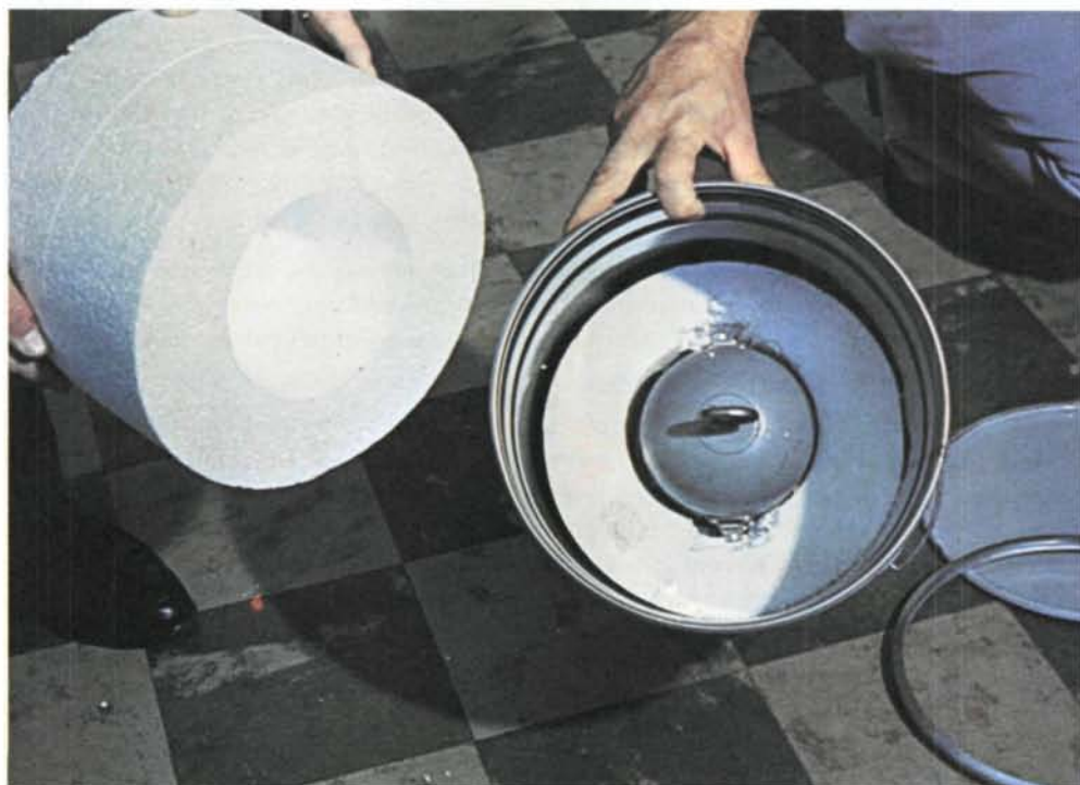
Figures 2a, 2b. Components and assembly of a Type A package of different design.
