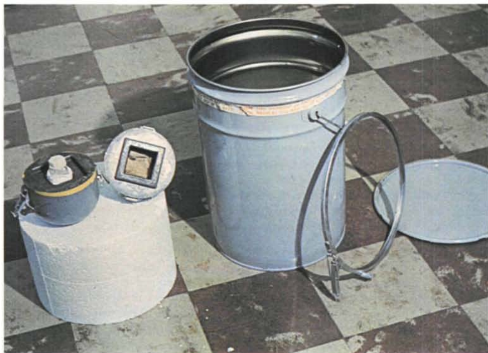
Figures 2a, 2b. Components and assembly of a Type A package of different design.
