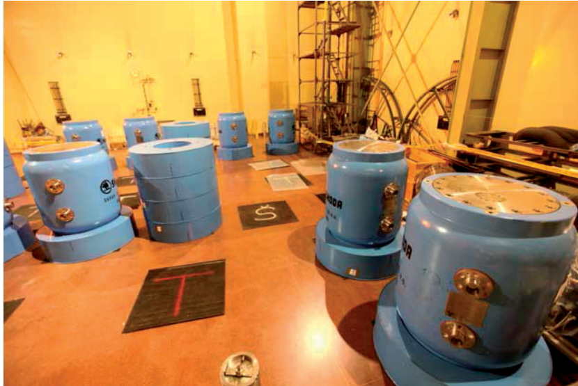
FIG. 22. Shipping cask operations in the reactor building at the Vinča site, Serbia.
