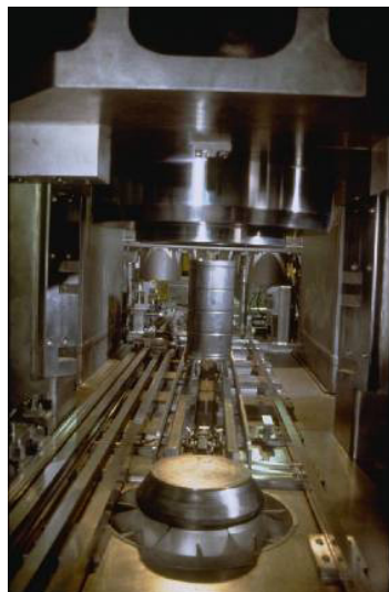
FIG. 2. Mock-up sheared fuel hull canisters (UC-C) (courtesy of AREVA).
