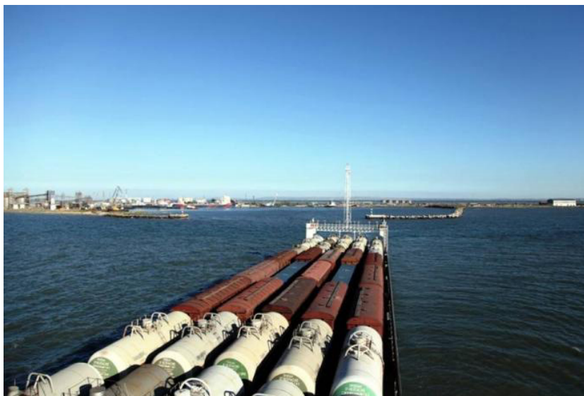
FIG. 21. First shipment of Class 7 dangerous goods by Anship LLC's ferry over the Black Sea from the port of Kavkaz (empty TUK-19 casks, UN 2907).
