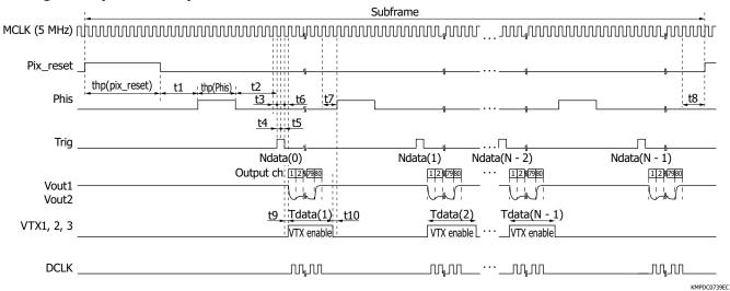
\*7: Data with different phase timing. One frame consists of four subframes (F1, F2, F3, F4).
