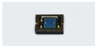
COB (chip on board)
