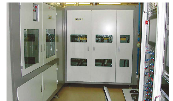
Thin-film crystal growth with MOCVD equipment
