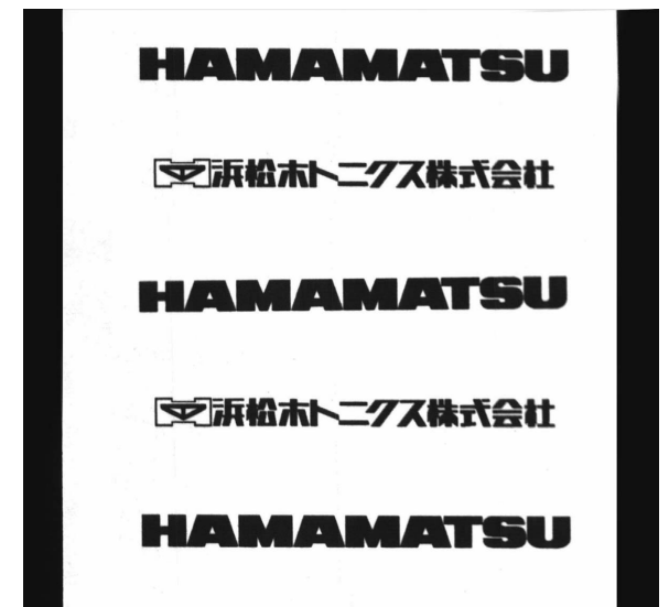
[Figure 1-24] Imaging in TDI operation (continuous image during drum rotation)
