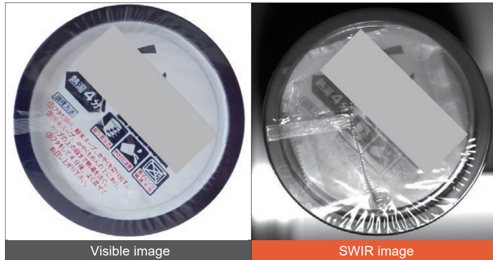
Sample: Instant noodles Wavelength: 1200 nm Illumination: Reflection
