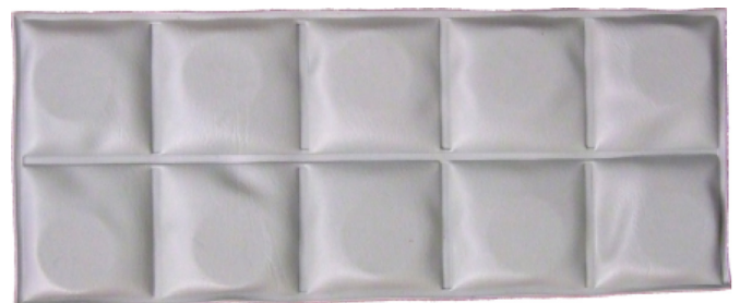
Simulation beta source for decontamination training
