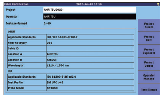
Cable Certification Test Conditions Screen
