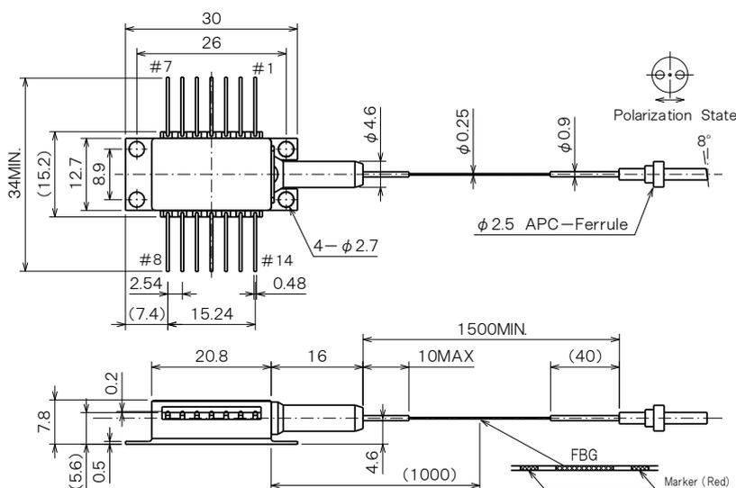
(Note) The polarization direction of the LD is parallel to the slow axis of the PMF.
