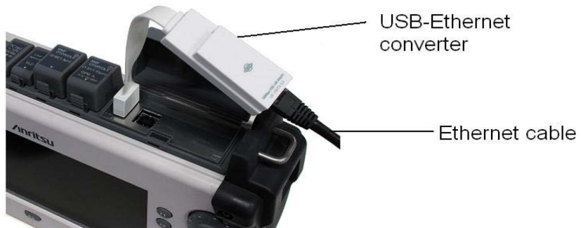
Figure 14-2: Ethernet Cable Connection
