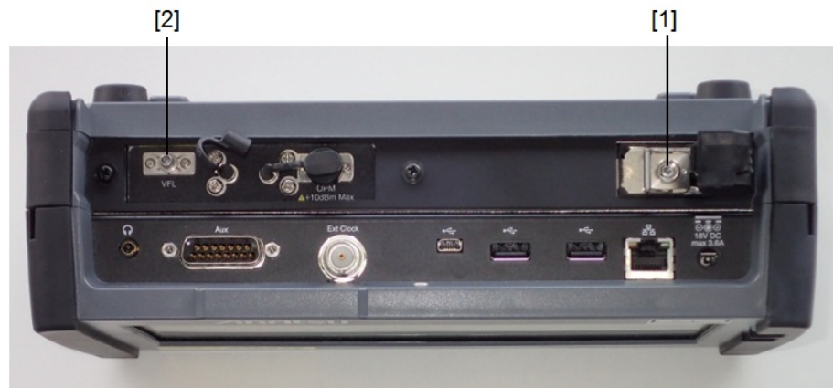
Figure 3: Locations of laser aperture (MU100022A)
