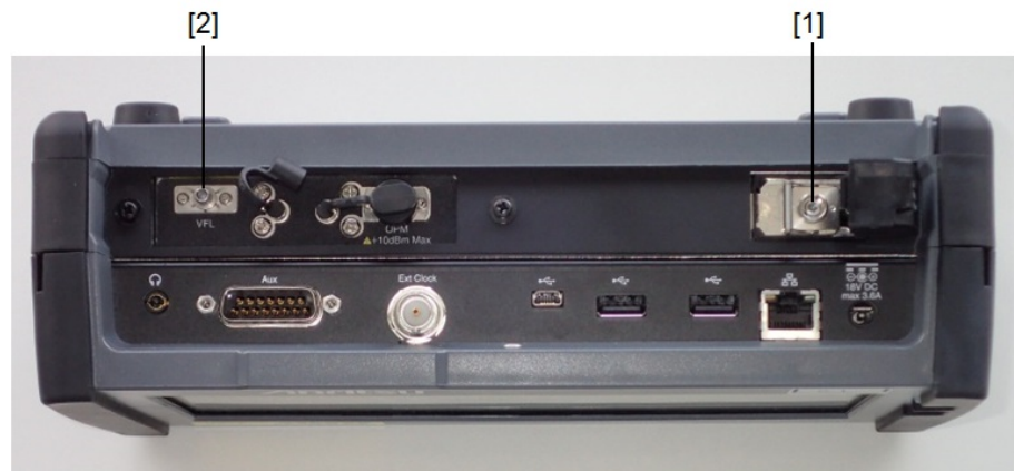
Figure 1: Locations of laser aperture (MU100020A)
