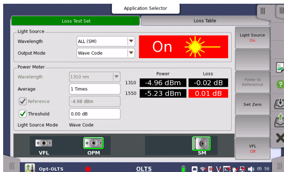
Receiving Light Modulated by Wave Code
