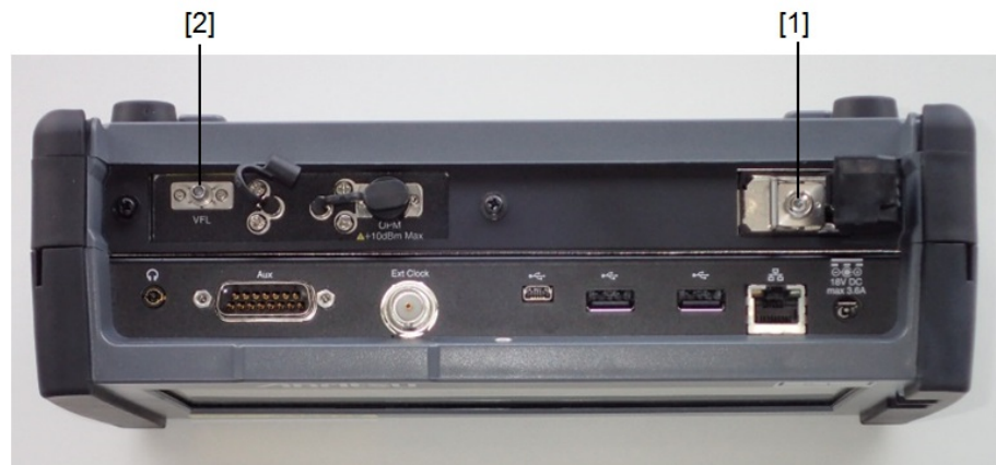
Figure 3: Locations of laser aperture (MU100022A)
