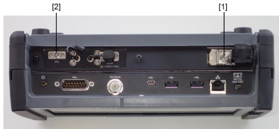
Figure 1: Locations of laser aperture (MU100020A)
