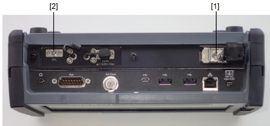
Figure 3: Locations of laser aperture (MU100022A)
