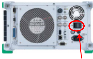
Main Power Switch
