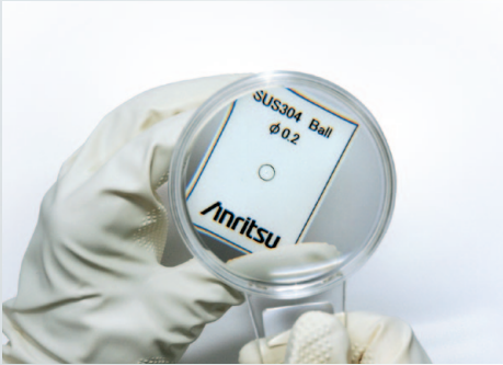
0.2 mm diameter sphere detectable
