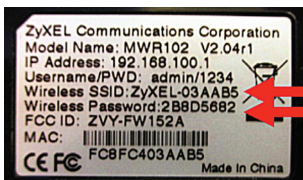
Figure 3. The Pocket Router configuration information.
