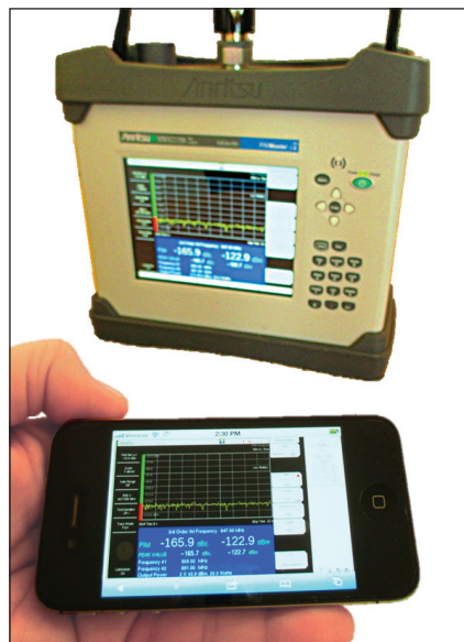
Figure 1. The PIM Master with wireless remote control via iPhone.
