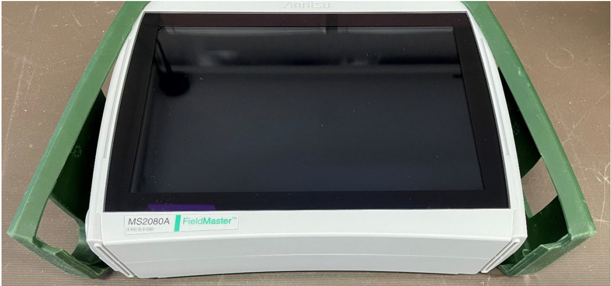
Figure 3-3. Pulling of Side Bumpers
