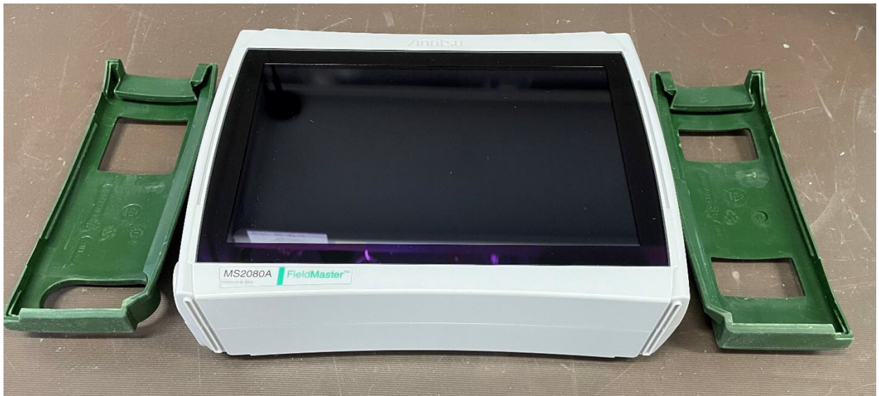
Figure 3-4. Side Bumpers Removal
