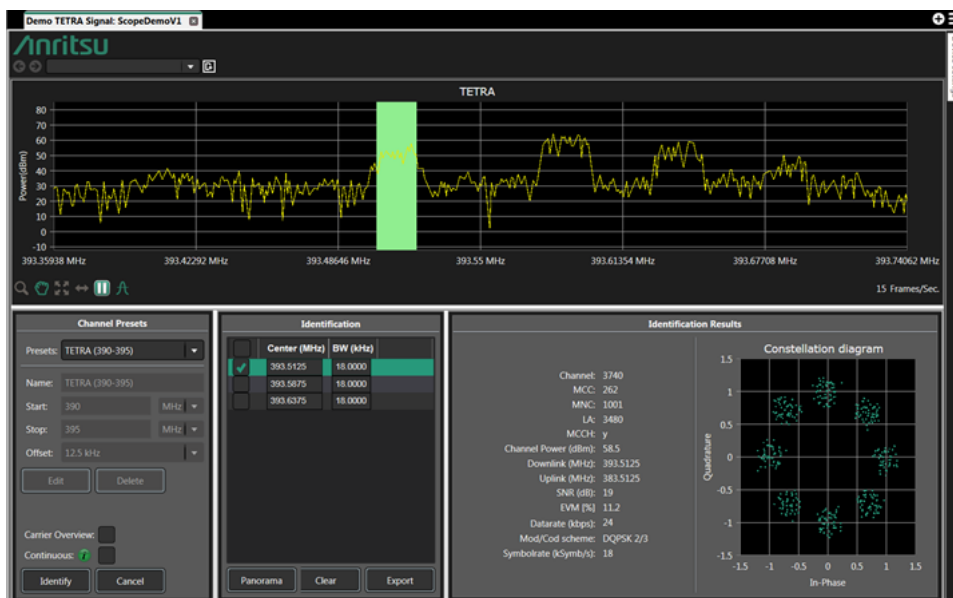
Figure A-5. Demo TETRA Signal: Demodulation Parameters and Constellation Diagram
