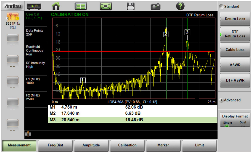
Figure 3-14. Failing DTF Return Loss Measurement (Antenna at 20.54 m)
