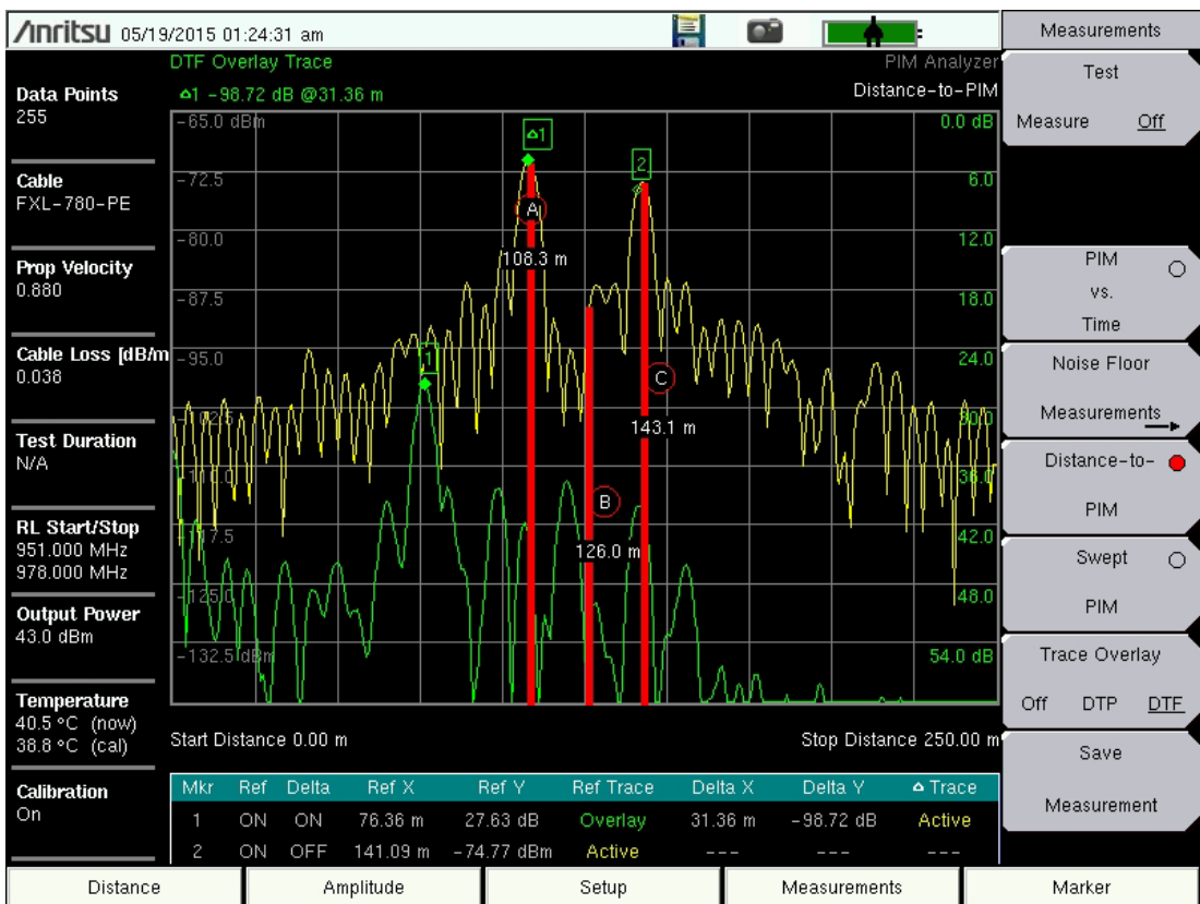
Figure 5-6. DTP/DTF Trace Overlay Example
