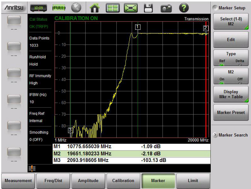
Figure 3-13. 2-Port Transmission Measurement Example, Waveguide
