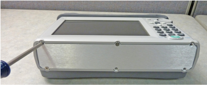
Figure 10-2. Remove the Battery Cover Plate
