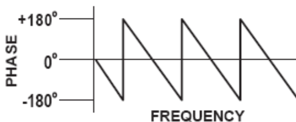
Figure A-15. Linear Phase with Frequency Waveform
