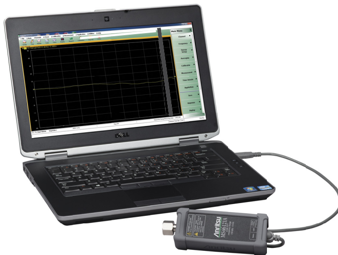
Figure 3-1. MS46121A/B Connected to the PC Controller
