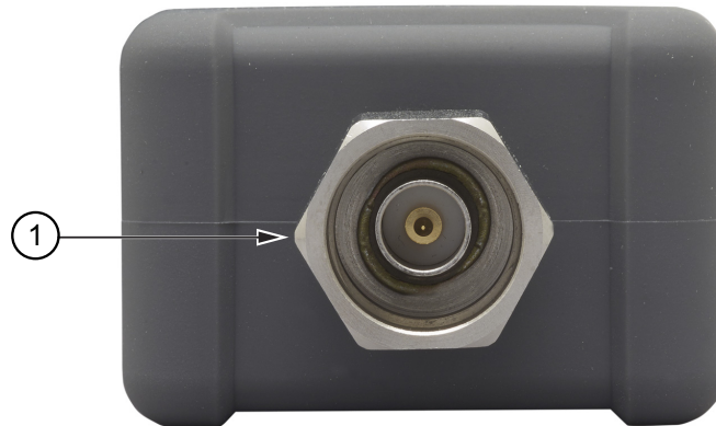
Figure 2-1. MS46121B N(m) Connector
