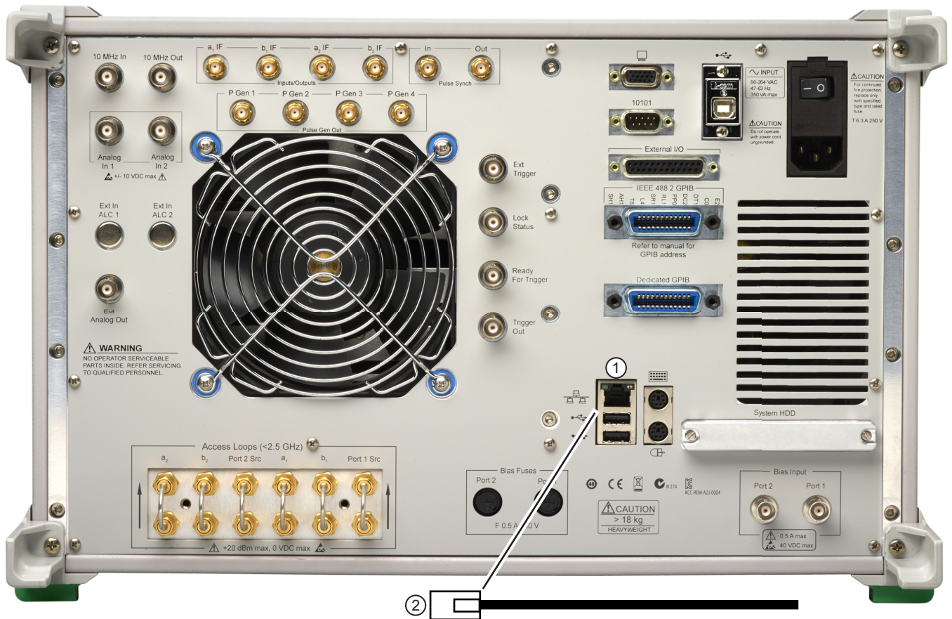
Figure 2-10. VectorStar MS464xB Series VNA Ethernet and USB Ports
