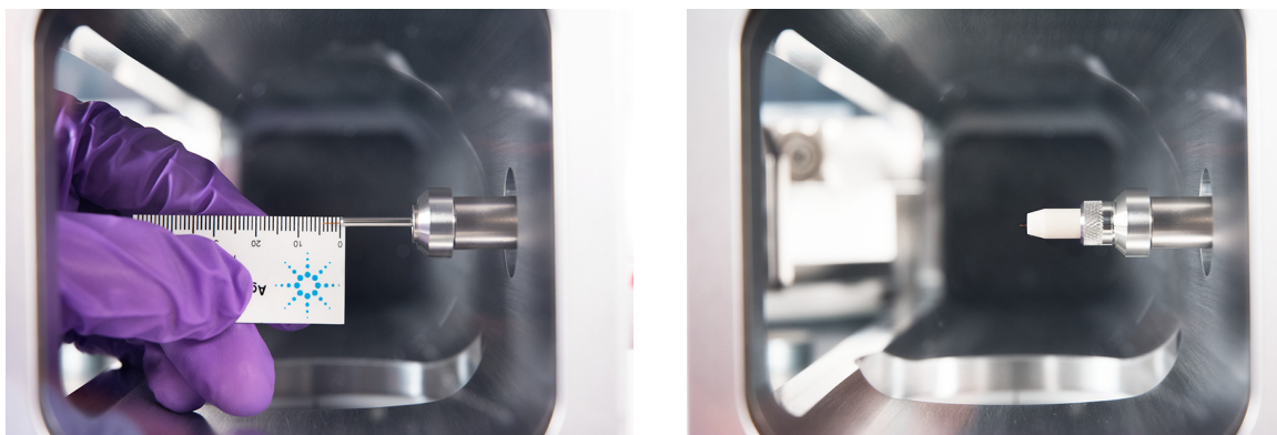
Figure 6. Installing a capillary column in the GC/MSD interface for an EI HES source.
