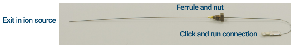
Figure 16. 9000 GC/MS Tail removed from GC/MSD Interface
