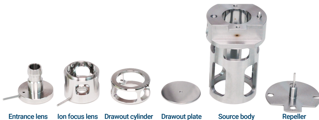
Figure 79. CI source parts to be cleaned
