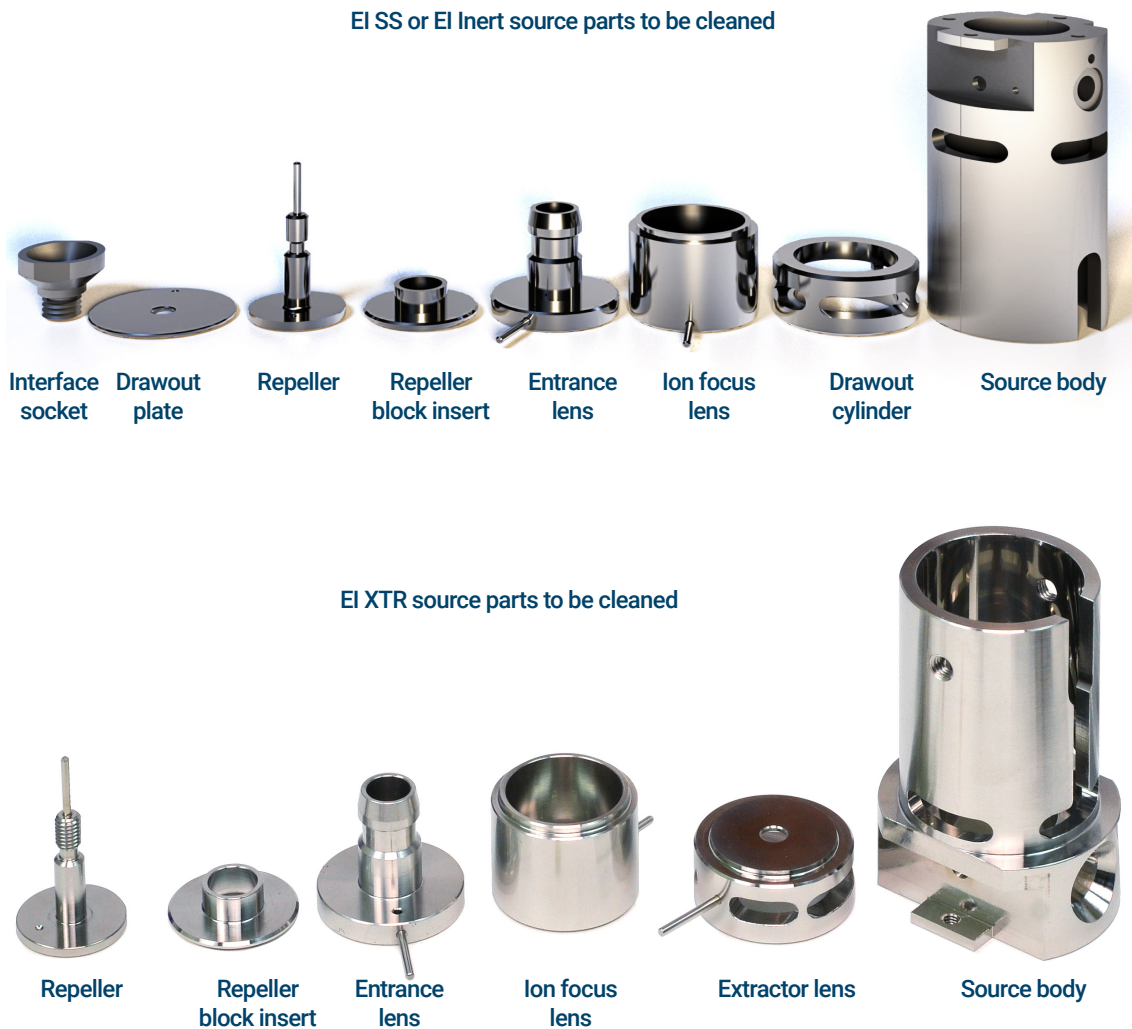
Figure 66. Source parts to be cleaned
