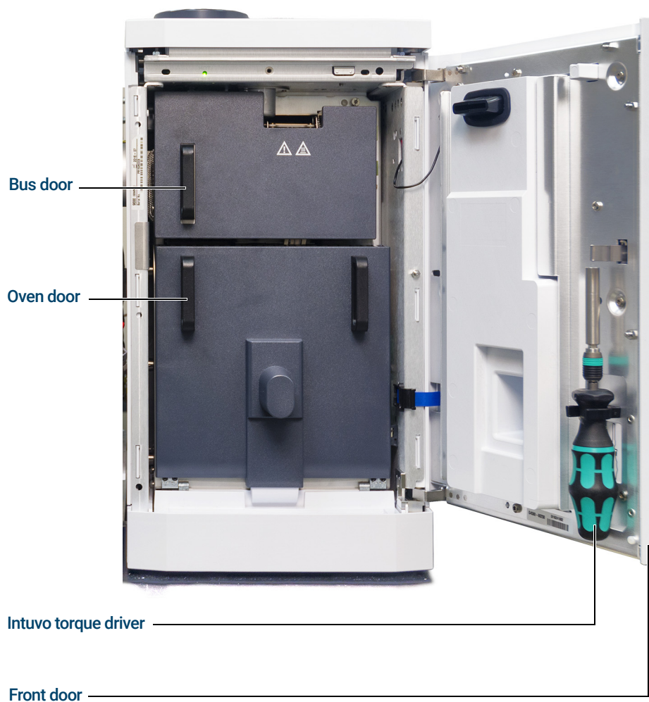
Figure 10. 9000 GC front door, bus door, oven door, and Intuvo torque driver
