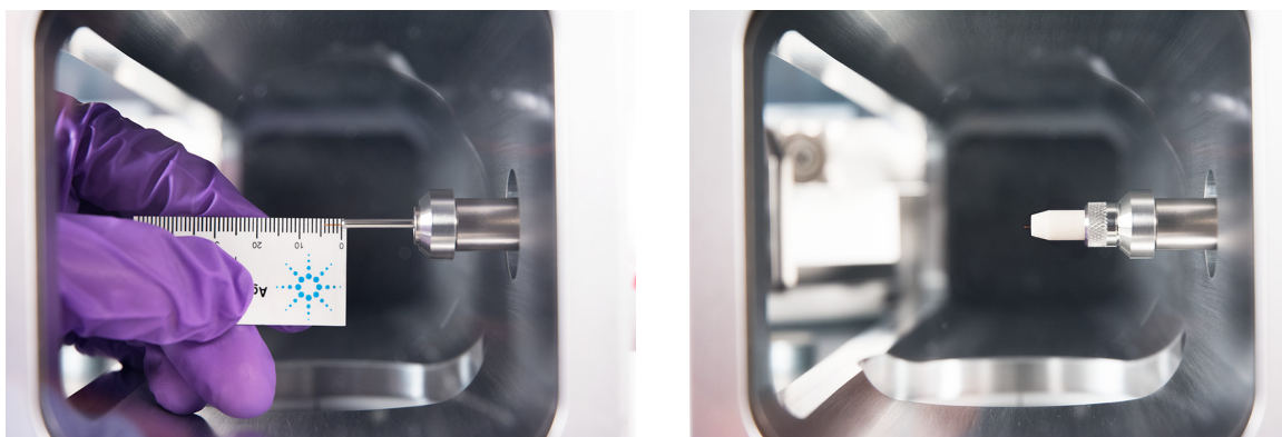
Figure 22. Installing a capillary column in the GC/MSD interface for an EI HES source.
