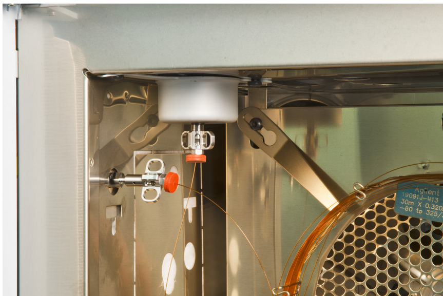
Figure 7. Installing a capillary column in the GC/MSD interface
