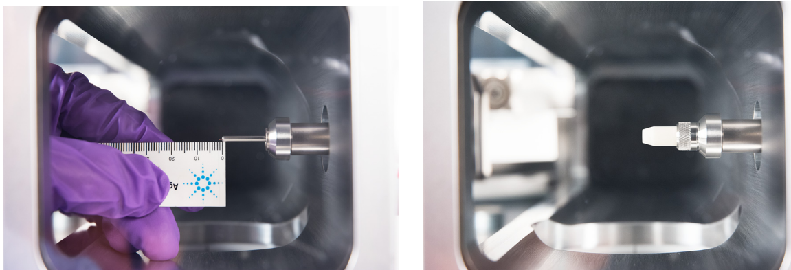
Figure 5. Installing a capillary column in the GC/MSD interface for an EI EXT, SS, Inert, or CI source.
