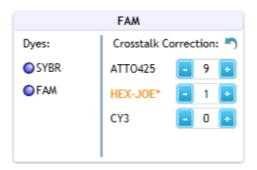
**2** Change the crosstalk correction setting for the dye by adjusting the value in the field.
