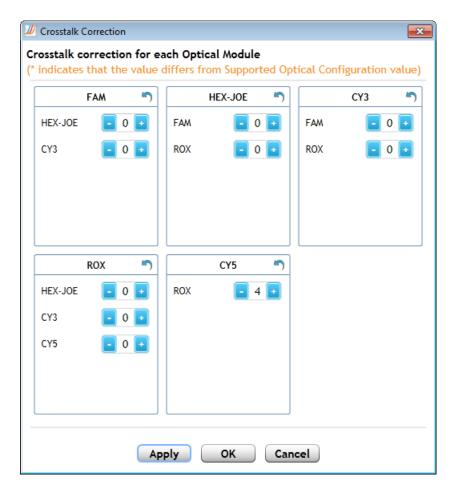
**4** In the dialog box, locate the box for the optical module that is reporting crosstalk fluorescence (i.e., the spillover optical module). The dyes that have the potential to crosstalk with that optical module are listed in that box (e.g., the ROX dye in the CY5 optical module).
