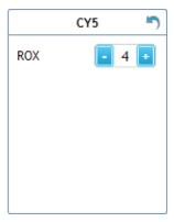
**5** Change the crosstalk correction setting for the dye by adjusting the value in the field.
