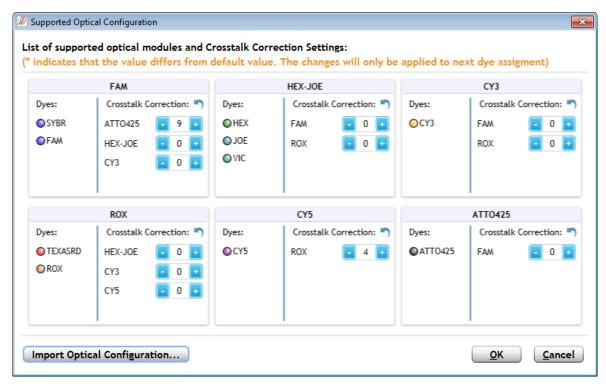
Crosstalk occurs when emission from one dye is detected by two different optical modules (the target optical module and the spillover optical module). A dye is at risk for crosstalk when its emission spectra overlaps that of another dye that is assigned to a different optical module. The Aria software includes crosstalk correction settings, which can help compensate for crosstalk.
