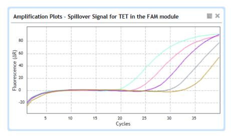
**3** Adjust the crosstalk correction setting for the spillover optical module until that optical module no longer detects an increase in fluorescence (i.e., the amplification plot for the optical module is as close to flat as possible in the graph). See instructions in "To adjust the crosstalk correction settings:" on page 204 for details on how to perform this step.
