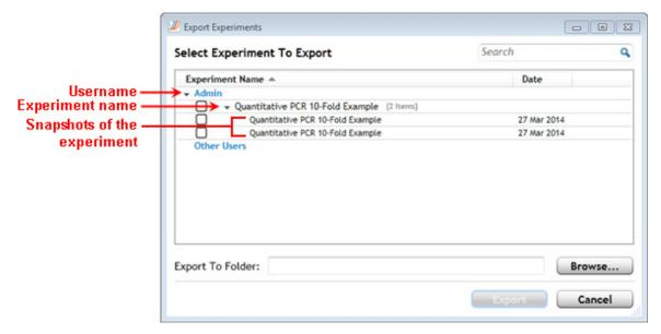
**2** Mark the check box for the experiment or snapshot that you want to export. Marking the experiment will export all snapshots of the experiment. Marking a snapshot will export only that snapshot. The date stamp for the snapshots are noted in the Date column.
