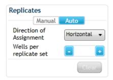
**3** In the **Direction of Assignment** drop-down list, specify how the replicate wells are arranged on the plate.
