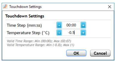
5 In the **Time Step (mm:ss)** field, add an increment to the duration of the plateau. The permitted range for the selected plateau (called the *Valid Time Range*) is displayed near the bottom of the Touchdown Settings dialog box. This range is based on the initial duration of the plateau and the number of cycles assigned to the segment. The maximum value for the range is designed to ensure that by the last cycle, the duration of the plateau does not exceed the maximum allowed duration.
