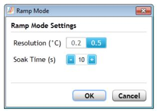
2 Next to **Resolution** (°C), select **0.2** to set the ramp to 0.2°C increments, or select **0.5** to set the ramp to 0.5°C increments.
