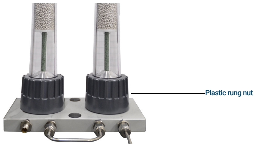
Figure 29. Tighten the plastic ring nut to secure the filter to the connecting unit
