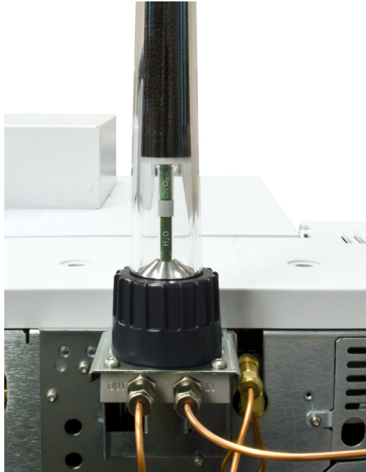
Figure 41. Unscrew the knurled or plastic ring nut
