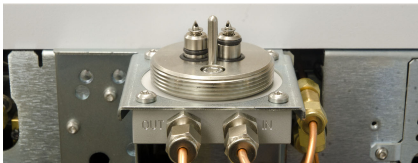
Figure 15. Bracket connecting unit installed on underside of bracket for PAL Auto Sampler configuration
