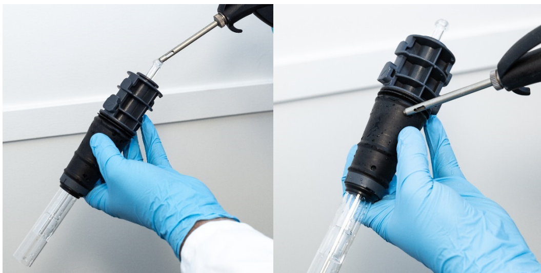
Figure 18A and B. Use compressed air, argon or nitrogen to dry the torch.
