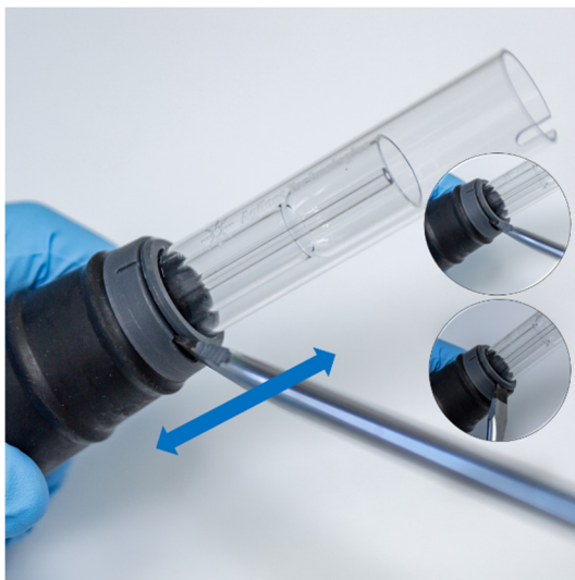
Figure 10. Removing the top seal with an aid of a wide blade flat screw driver
