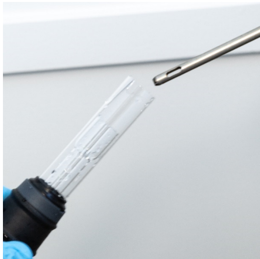
Figure 19. Blow clean compressed air, argon or nitrogen through the open end of the tube-set.
