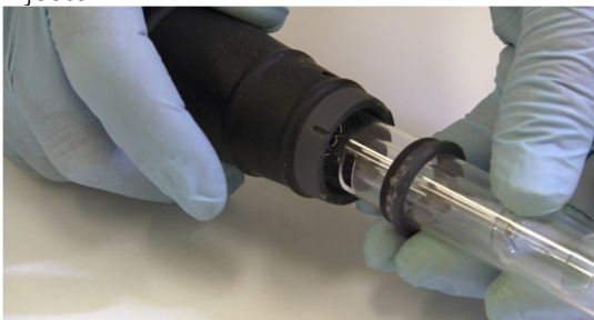
Figure 6. Torch inserted into torch body
