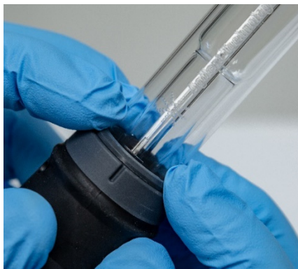
Figure 8. Ensure the seal is properly seated by pressing firmly on the top edges
