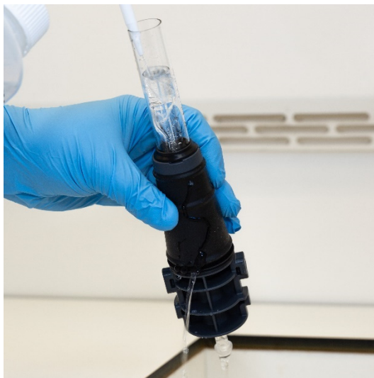
Figure 16B. Flush the gas ports and ball joint connector with deionized water.
