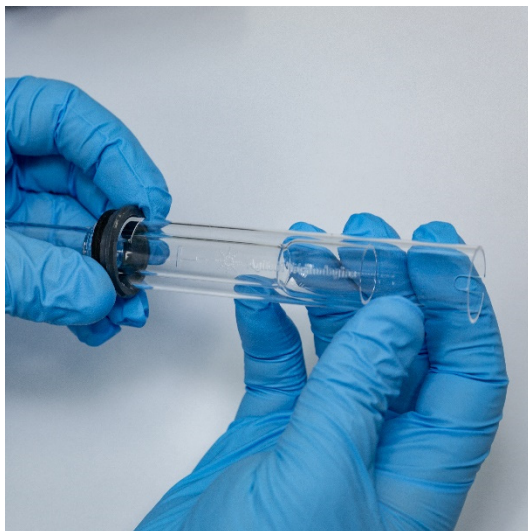
Figure 4. The top seal being refitted to the quartz outer tube-set
