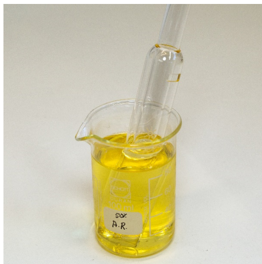
Figure 15D. Quartz outer tube-set soaking in aqua regia.
