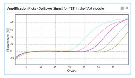
**3** Adjust the crosstalk correction setting for the spillover optical module until that optical module no longer detects an increase in fluorescence (i.e. the amplification plot for the optical module is as close to flat as possible in the graph). See instructions in "To adjust the crosstalk correction settings:" on page 182 for details on how to perform this step.
