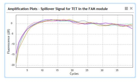
**4** For all experiments that include this dye, make sure that the crosstalk correction setting for the spillover optical module is set to the value determined in Step 3 above. To change the default crosstalk correction settings for future experiments, see "Change the default crosstalk correction settings" on page 26.
