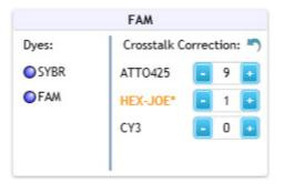
**2** Change the crosstalk correction setting for the dye by adjusting the value in the field.
