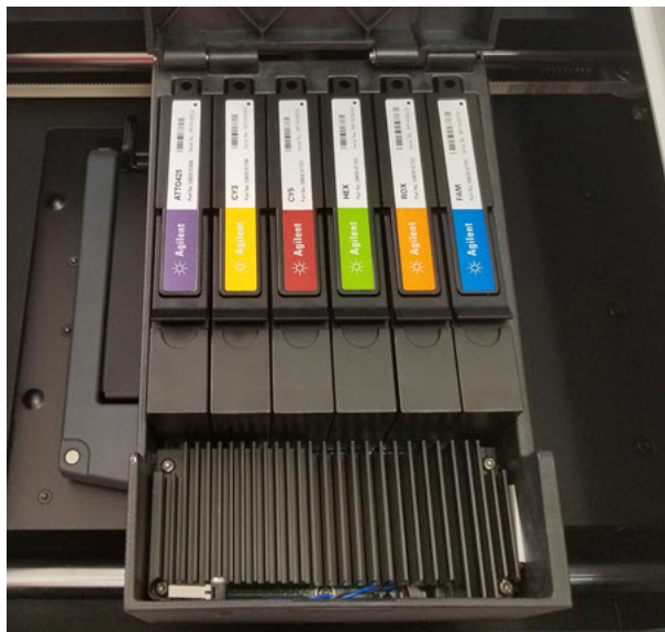
Figure 10 Installed optical modules
