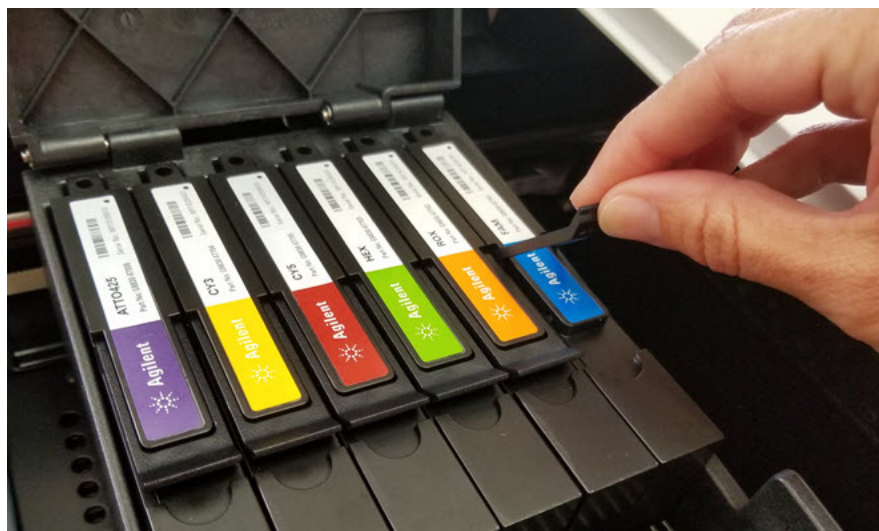
Figure 47 Lifting the hinged tab on an optical module
