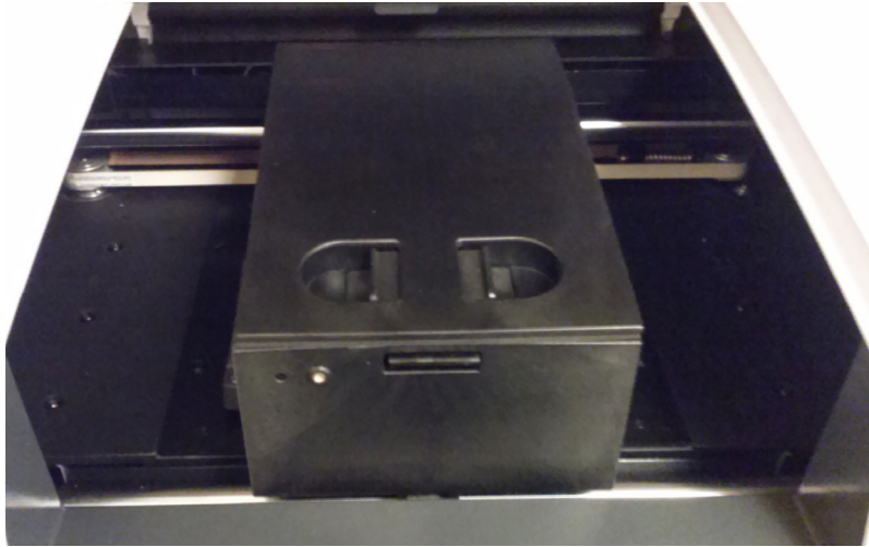
Figure 5 Optical module housing carrier, centered in the instrument door opening
