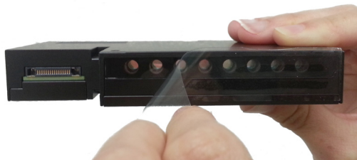
Figure 9 Removal of plastic film from optical module
