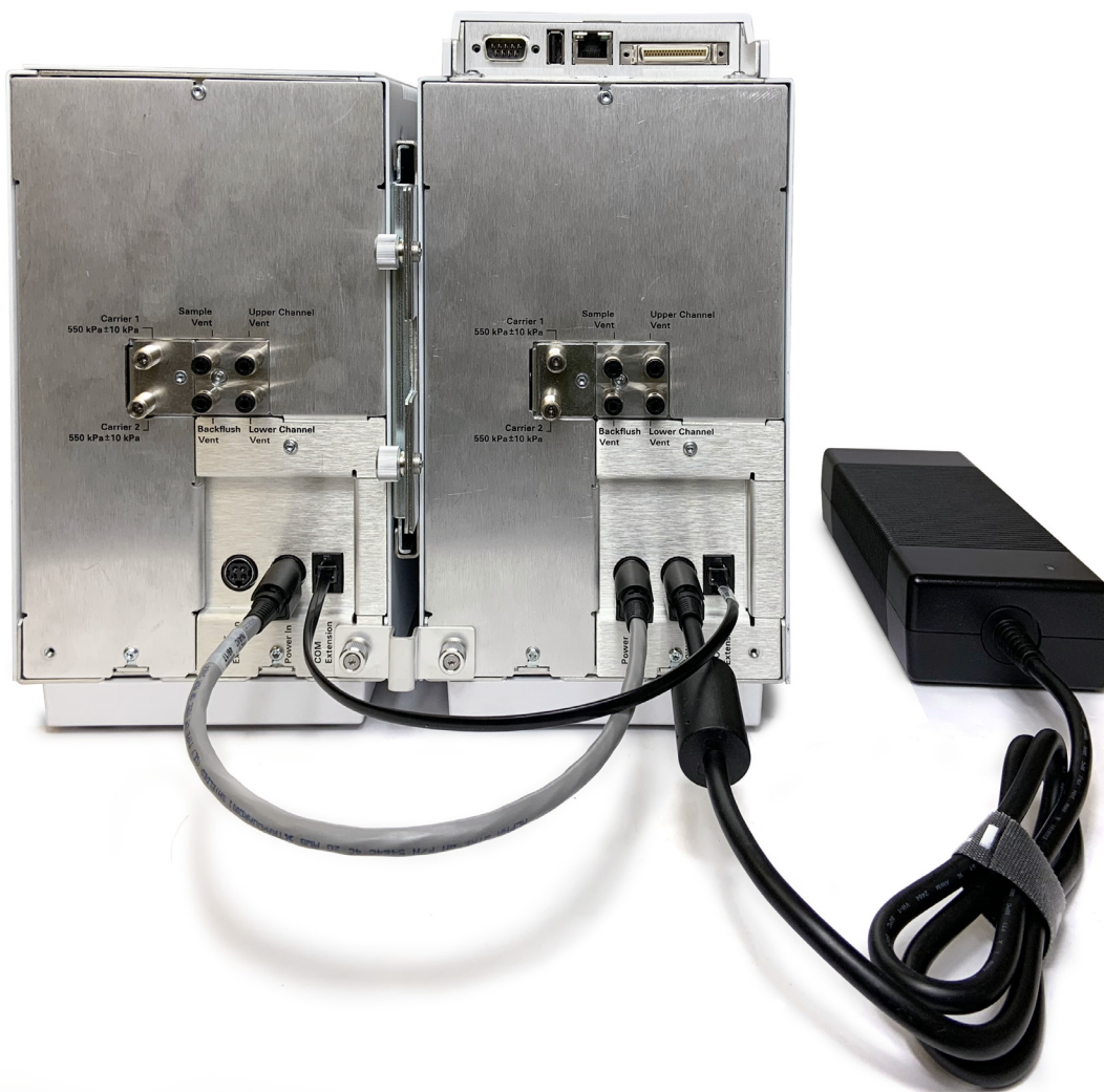
Figure 11. Rear view of two GC channel cabinets connected
