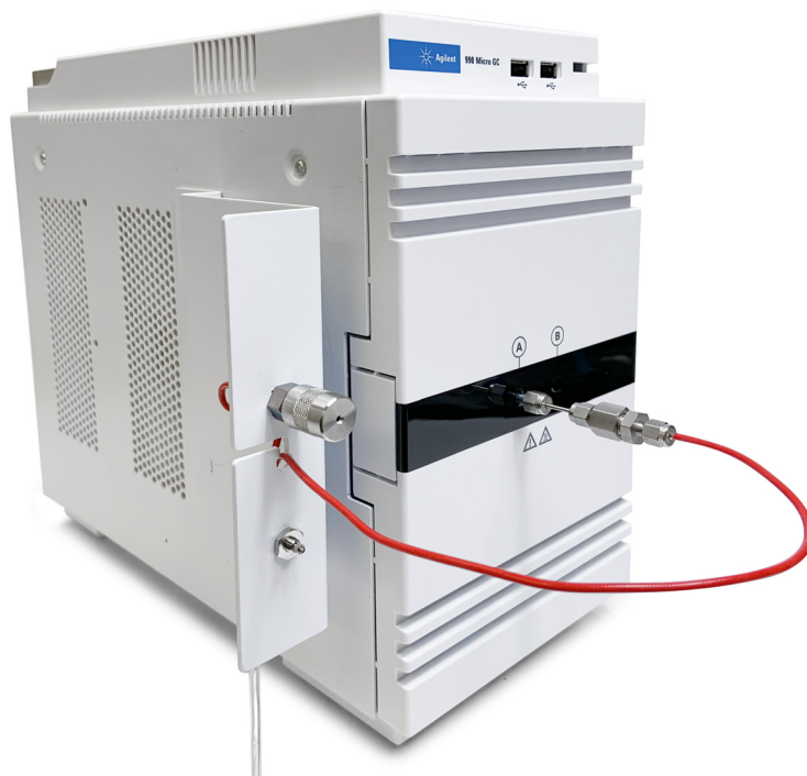
Figure 20. Septum nut injection port (p/n G3588-68865) installed
