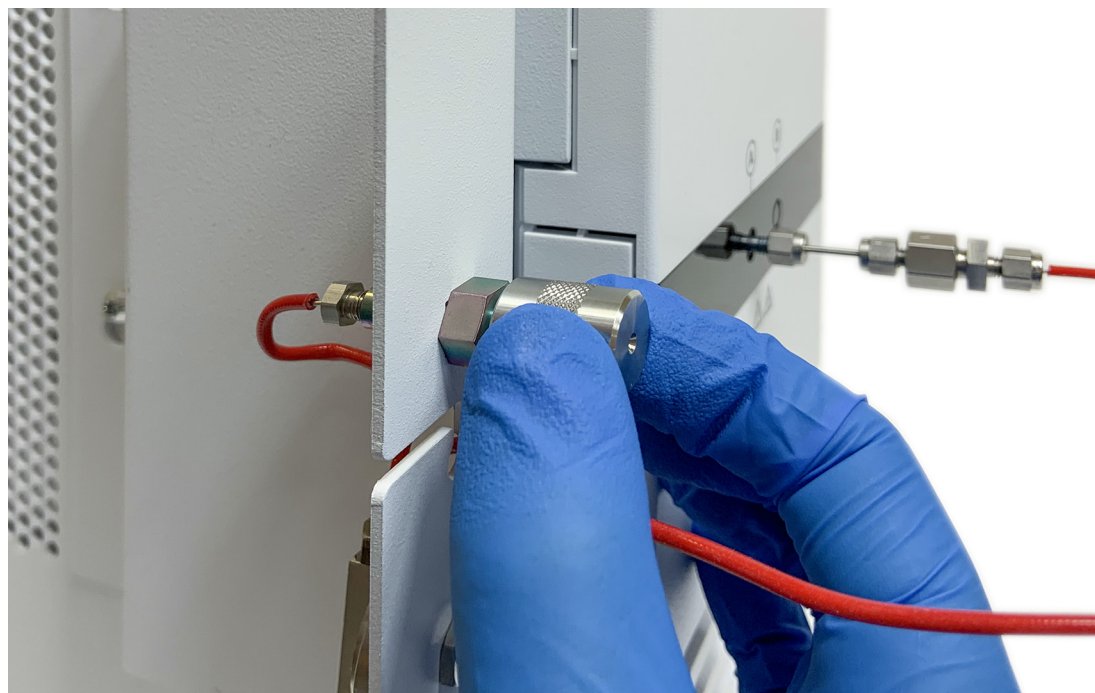
Figure 38. Manual injection septum replacement
