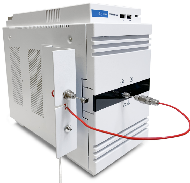
Figure 21. Luer lock injection port (p/n G3588-68866) installed
