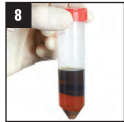
8 Phase separation of acetonitrile and aqueous layer
