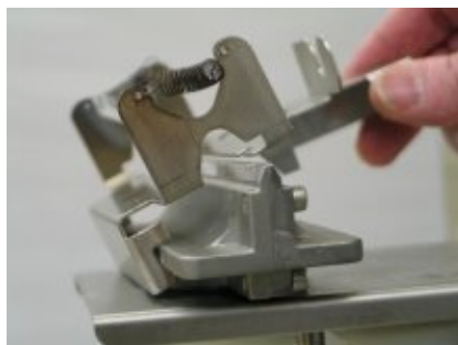
Figure 7. Cell holder pulled forward with cut-outs hooked around burner edge
