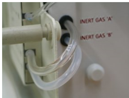
Figure 3. Inert gas tubing from pump unit correctly connected to nipples on reagent manifold
