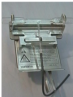
Figure 15. Mark 7 burner with standard absorption cell in cell holder positioned on top
