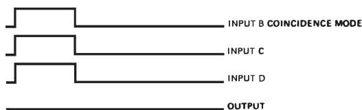
Coincidence Requirements When Switch Setting is 4.
