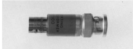
IT100 Inverting Transformer A compact pulse-inverting transformer for use in a 50- \Omega system; has low distortion; good linearity, freedom from overload effects, 0.8-ns rise time capability, and 7% tilt in 100 ns.
