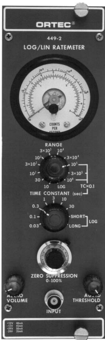
The ORTEC Model 449 is the same module as shown, except that it has no audio volume or threshold control.
