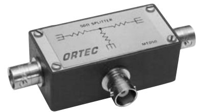
MT050 50- \Omega Matched Tee Signal Splitter One input provides two equal half-amplitude outputs and still preserves 50- \Omega termination; reflection, typically 10% (dc to over 500-MHz equivalent bandwidth); rise time, 1 ns; continuous input power, 1 W.
