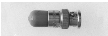
T50 Terminator, 50 \Omega , BNC. Provides a high-quality 50- \Omega ( \pm 1\% ) 1/2-W termination.
