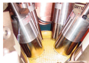
Four Detector ACTINIDE-85 Array for Lung Burden Measurements.
