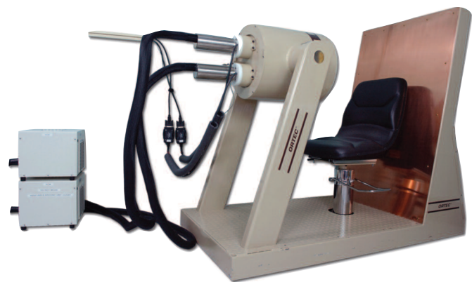
Dual HPGe Detector System with X-COOLER III.
