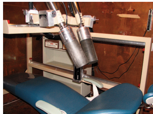
Low-Background Room with Whole-Body Counting Detectors Cooled with X-COOLER III units.
