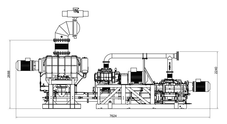
Note: this is an example of a typical steel degassing module system for VD applications. Edwards systems can be adapted for individual customer requirements
