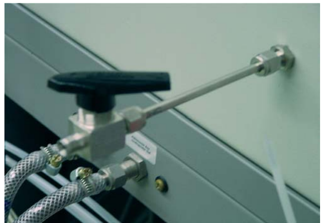
Feedthrough DN 10 with Swagelok handvalve
