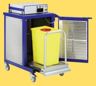
For radionuclides like <sup>11</sup>C, <sup>18</sup>F, <sup>57</sup>Co, <sup>90</sup>Sr, <sup>99m</sup>Tc, <sup>111</sup>In, <sup>125</sup>I or <sup>131</sup>I in typical waste containers filled with low density waste detection limits below 0.2 Bq/g can be achieved within a few minutes.
