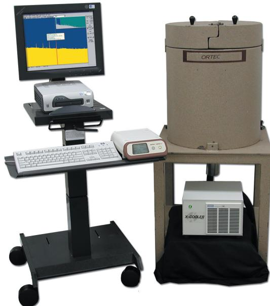
DSPEC LF is the third and newest member of the DSPEC USB family of digital technology gamma ray spectrometers from ORTEC. It provides the same rock solid spectral stability with variation in temperature and count rate and retains many of the valuable attributes of the other two models. Many environmental and radiochemistry laboratories will find this instrument to be the best MCA for day-to-day sample counting with laboratory HPGe or NaI detector systems.
