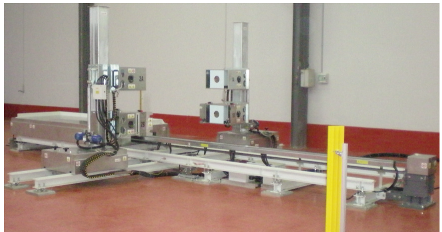
General view of sample platform showing the mounting of the two IDMs and collimators on either side of the measurement zone through which the container passes.
