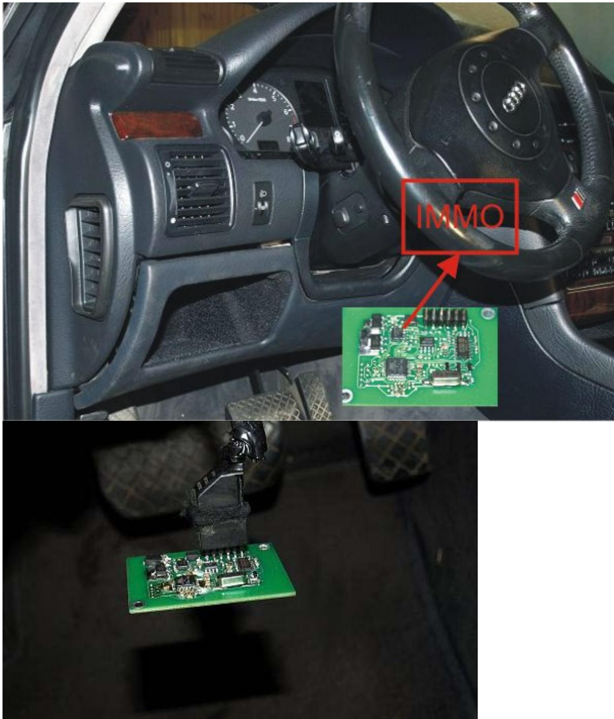
After emulator is installed to car switch ignition on/off with all valid keys you have keys will be programmed in automatically
