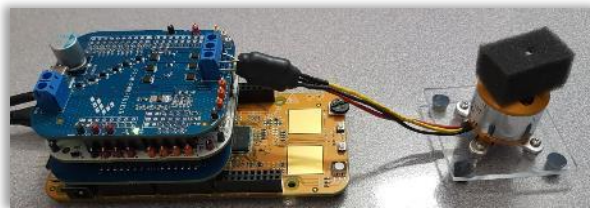
BLDC Motor Control S32K144 + GD3000
