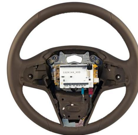
1. Sensitivity tuned for 2mm plastic glass overlay on a top of the electrodes (3mm available)
