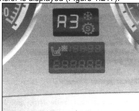
Fig. 1.217. Indicator boxes Easytronic transmission
